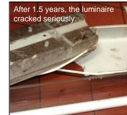
After 1,5 years, the luminaire cracked seriously.
